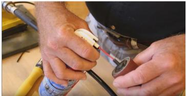
An alternative way to fill the Kirjes drums is with an air spray can.
