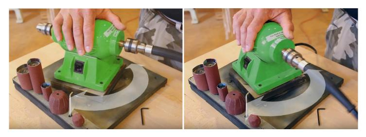
When mounting the Kirjes motor on a rotating plate it will be easier to work with the flexible shaft, especially when working with larger pieces.
